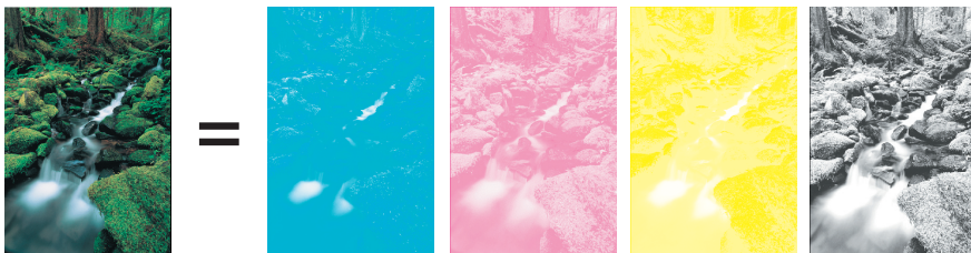
Process Color Separations. 4 plates: cyan, magenta, yellow and black produce a full color effect.
